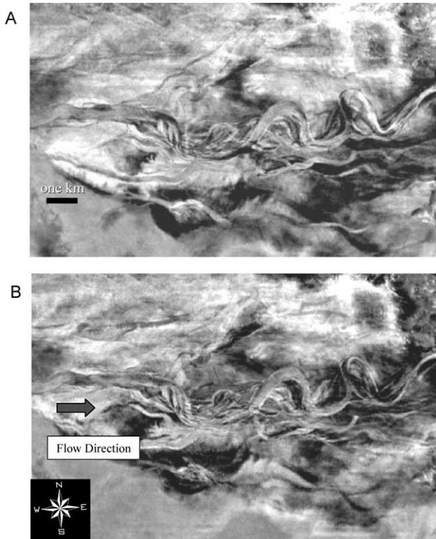
Fig. 19. Moderate to high-sinuosity channel at the top of the frontal splay deposit illustrated in Fig. 18. This channel is characterized by down-system meander loop migration.
