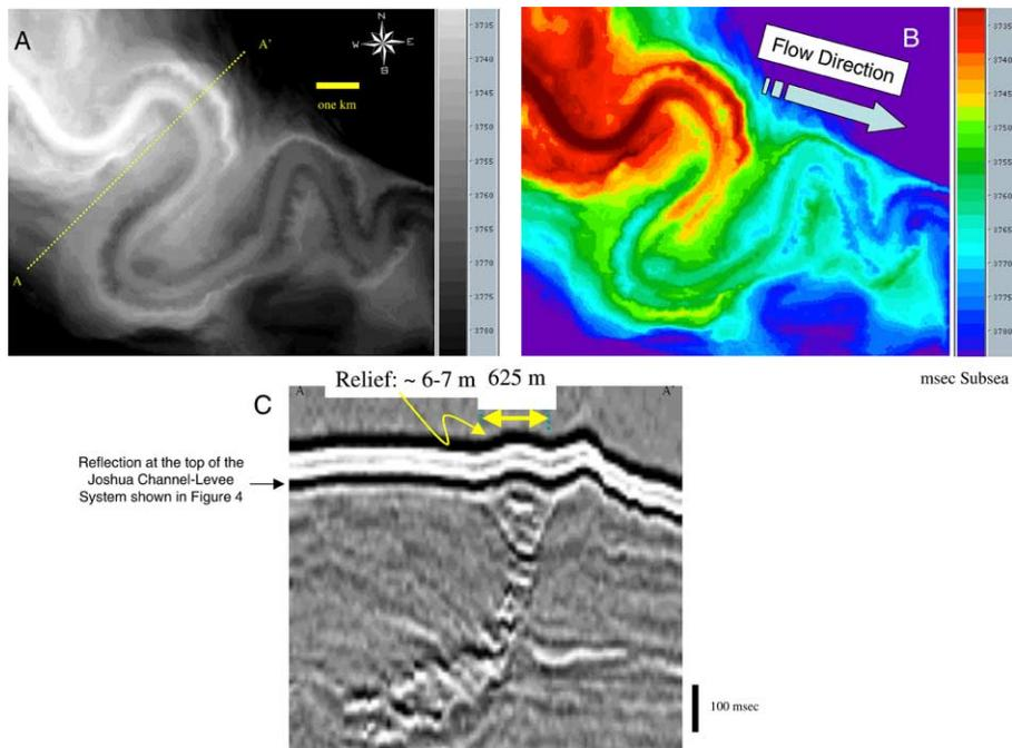
Fig. 5. Black and white (A) and color (B) time structure maps of the upper bounding surface of the Joshua channel-levee system (location shown in Fig. 4). (C) Transverse seismic reflection profile across the leveed channel illustrating 6–7 m of relief associated with the channel fill and similar relief associated with the levee. The high amplitude reflections that characterize the channel fill suggest a sand prone amalgamated aggradational fill architecture.
