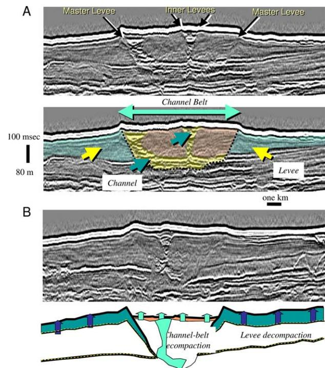
Fig. 12. (A) Transverse seismic reflection profile across the Joshua channel belt and associated levees. The master bounding levees as well as the levees bounding the Joshua channel are shown. The channel is inferred to be most sand prone, followed by the channel belt, which is less sand prone, and the overbank, which is least sand prone. (B) illustrates the decompacted configuration of the leveed channel system.
