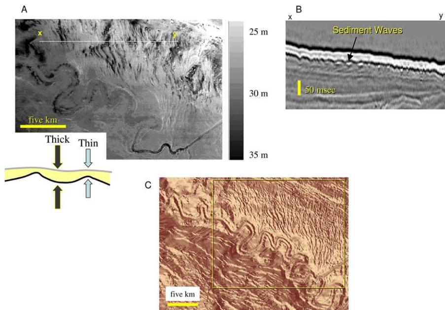
Fig. 16. (A) Time-thickness map between sea floor and the upper bounding surface of the Joshua channel-levee system. Varying thickness of this section suggests that these deposits represent progressive passive infill of low areas rather than continued active sediment wave aggradation or drape. (B) Seismic reflection profile oriented normal to long axes of sediment wave field illustrating the fill geometry of this overlying section. (C) Dip azimuth map of top of Joshua channel-levee system.
