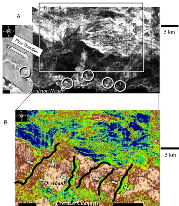
Fig. 17. Horizon slice illustrating five avulsion nodes with associated avulsion channels. The amplitude brightening on either side of the avulsion channels suggests the presence of sand there. The western-most avulsion channel feeds a frontal splay. This feature is characterized by numerous small channels.
