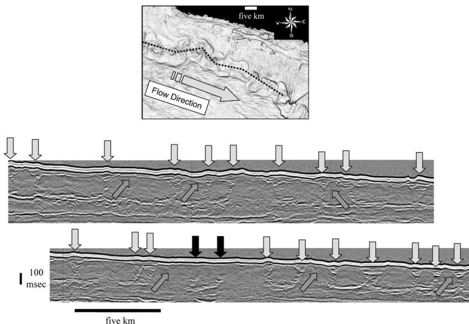
Fig. 8. Axial seismic reflection profile through the channel belt. Arrows indicate channel crossings. The black arrows indicate an abandoned meander loop. Sixteen of the channel crossings are characterized by down-system meander loop migration. One abandoned channel segment is shown.
