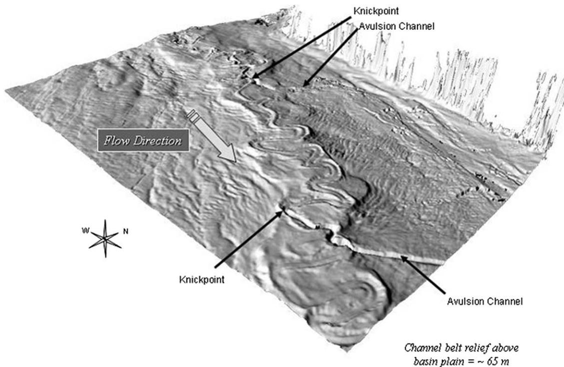
Fig. 13. Three-dimensional perspective view of the Joshua channel belt. The channel belt can be seen to lie above the adjacent levee. Two knickpoints are indicated. Note that the channels are concave-up troughs down-system from each knickpoint and the knickpoints mark the transition from concave-up to convex-up channel character. For scale, note that the convex up Joshua channel fill is approximately 625 m wide.
