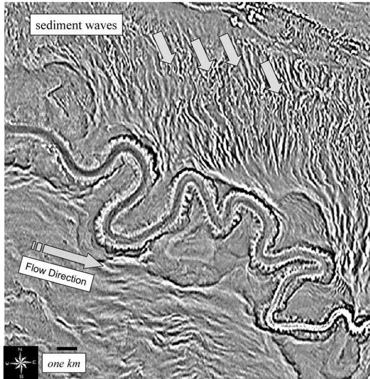
Fig. 15. Curvature map of upper bounding surface of Joshua channel-levee system. Depositional elements shown include overbank sediment waves, channel, channel belt, and slump scars on the inner flank of the levee. Arrows indicate sediment waves.
