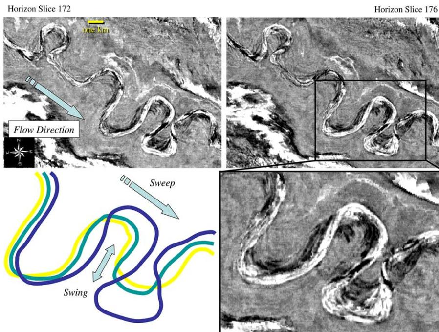
Fig. 9. Detail of the Joshua channel illustrating meander loop expansion (swing) and meander loop down-system migration (sweep). The line drawing of the channel locations illustrates the order of channel formation with yellow being the oldest position and purple being the youngest.
