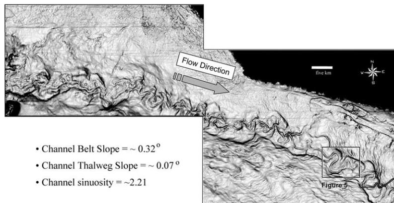
Fig. 4. Dip magnitude map of the upper bounding surface of the Joshua channel-levee system (see Fig. 5 for seismic reflection profile with this surface identified).
