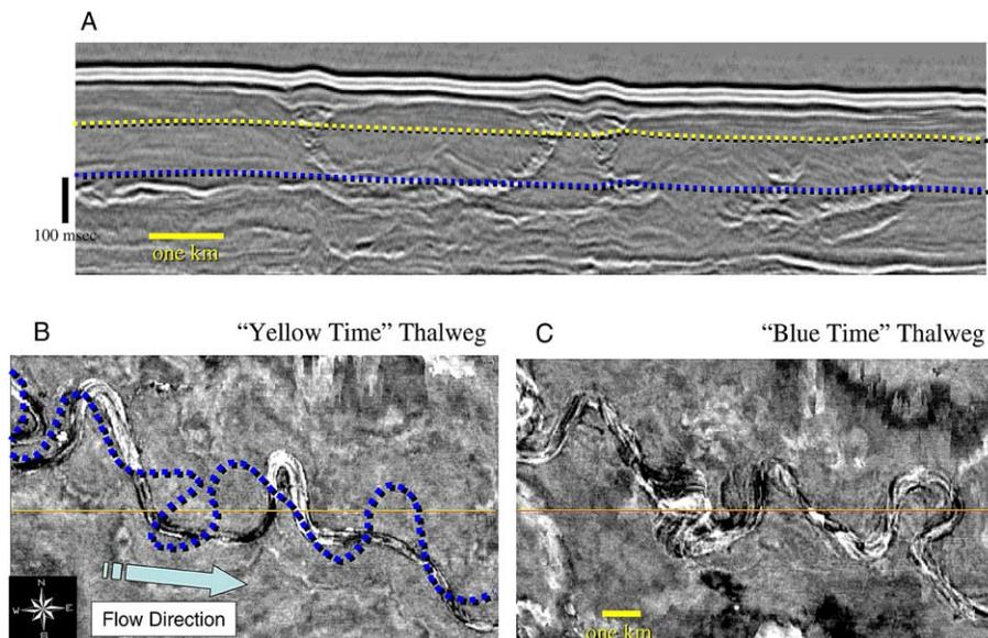
Fig. 10. (A) axial transect through the channel belt. A horizon slice at the upper dashed line (B) and the lower dashed line (C) illustrates the extensive shift in position of the channel axis through time. Part C also illustrates the tendency towards down-system meander loop migration (i.e. sweep).
