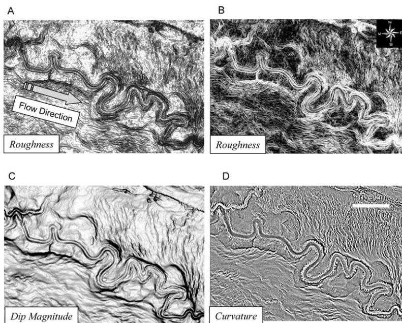
Fig. 6. Detail of the Joshua channel. Roughness (A and B), dip magnitude (C), and curvature (D), maps are based on analysis of 75 m<sup>2</sup> areas. The roughness maps are reverse polarity images of each other. Sediment waves, the convex-up aspect of the channel, and scoop-shaped slump scars can be observed to varying degree on these images.
