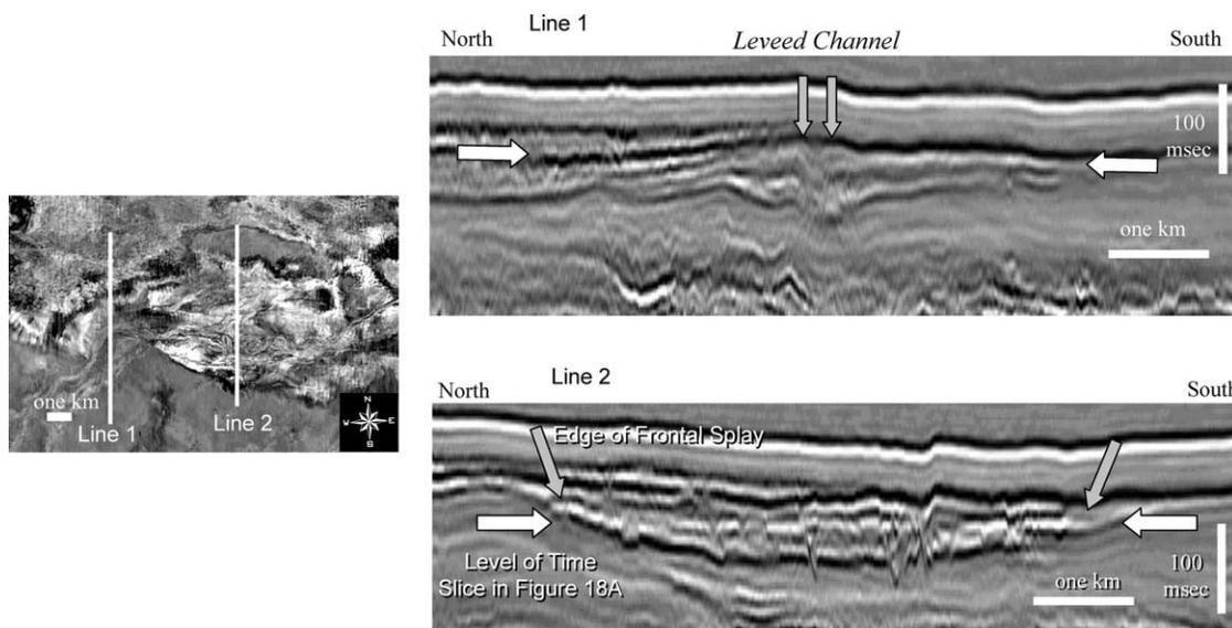
Fig. 18. Seismic reflection profiles oriented transverse to avulsion channel (A) and frontal splay (B). Note the numerous channels that characterize the frontal splay (B). Location shown in Fig. 17.
