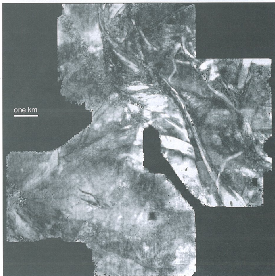
Fig. 4. Negative polarity total amplitude of 16 ms thick seismic interval bracketing a fluvial/deltaic depositional environment. Crosscutting channels give indication of temporal relationships; eight discrete levels of channels can be observed.
