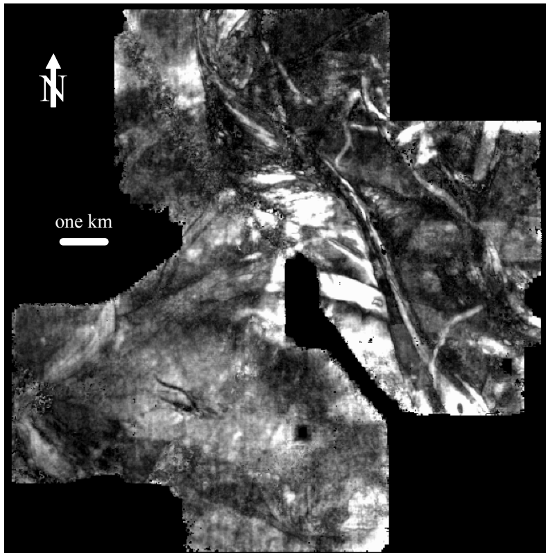
Figure 5. Network of Cretaceous channels, southern Alberta, imaged on amplitude extraction from seismic horizon slice. Channel edges are well defined in response to sharp lithologic contrasts that characterize the channel fill/over bank contact. The timing of channel formation can be determined from analysis of cross-cutting relationships.
