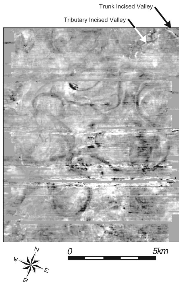
**Figure 8.** Detail of unincised alluvial geomorphology at time slice 112 ms subsea (location shown in Figure 2). Note the numerous meandering channels and that no incised tributary valleys are associated with these channels.
