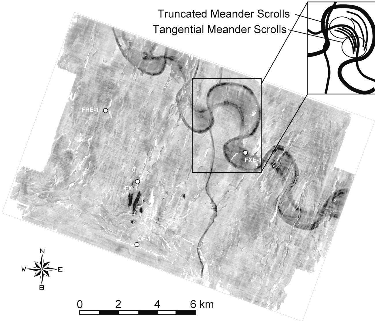
**Figure 16.** Seismic horizon slice through 3-D seismic volume at FXE area. Two channels can be observed. The high-sinuosity channel flow direction is to the southeast, and the low-sinuosity channel flow direction is to the south. Note the scroll bars in the meander loop just to the north of well FXE-1; they appear to be truncated to the northwest and tangential to the southeast.
