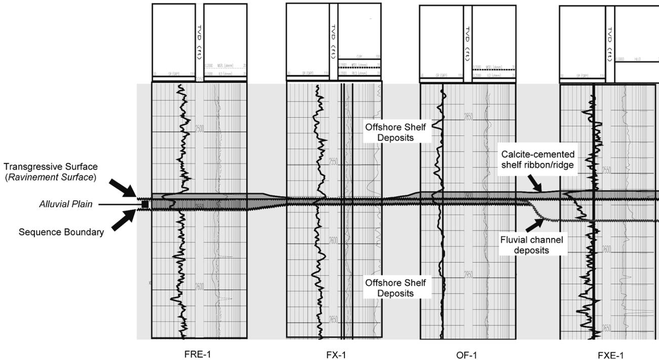
**Figure 17.** Well-log cross section from FXE area showing unincised lowstand alluvial system and associated flood plain embedded within offshore shelf sediments. A thin calcite-cemented zone inferred to consist of shell fragments in a siliciclastic sand matrix overlies the alluvial deposits.
