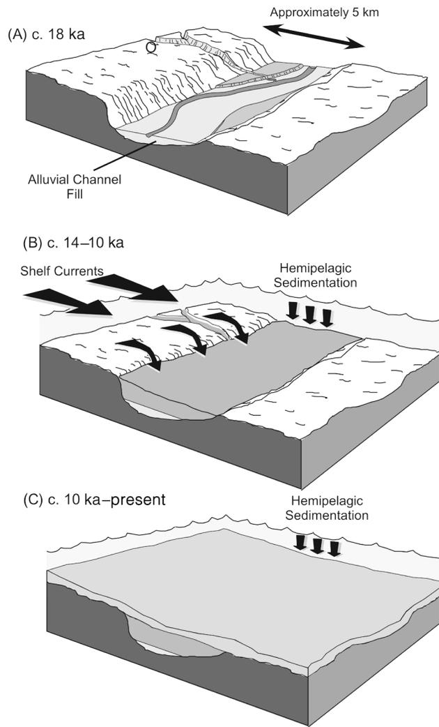
**Figure 12.** Schematic depiction of the evolution of incised valley fill in the Northwest Corner area from the time of maximum sea level lowstand, characterized by fluvial deposition (A), through the time of rapid transgression and filling by traction and hemipelagic sedimentation (B), and finally the time of sea level highstand and deposition of hemipelagic drape over the entire area (C).
